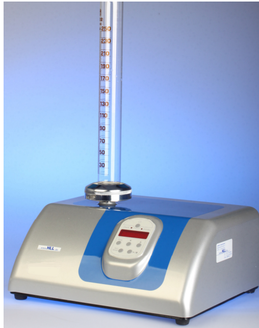
Tap density apparatus L5293307 and measuring cylinder L5293307M
