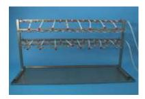
Temperature control unit with hose connection of 17 separating funnels 51816001t
